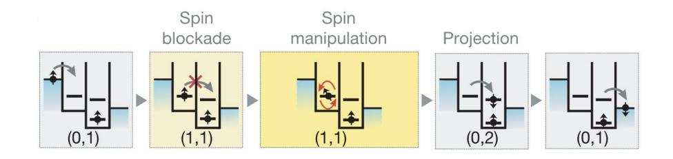
Triplet blockade: spin-to-supercurrent conversion
